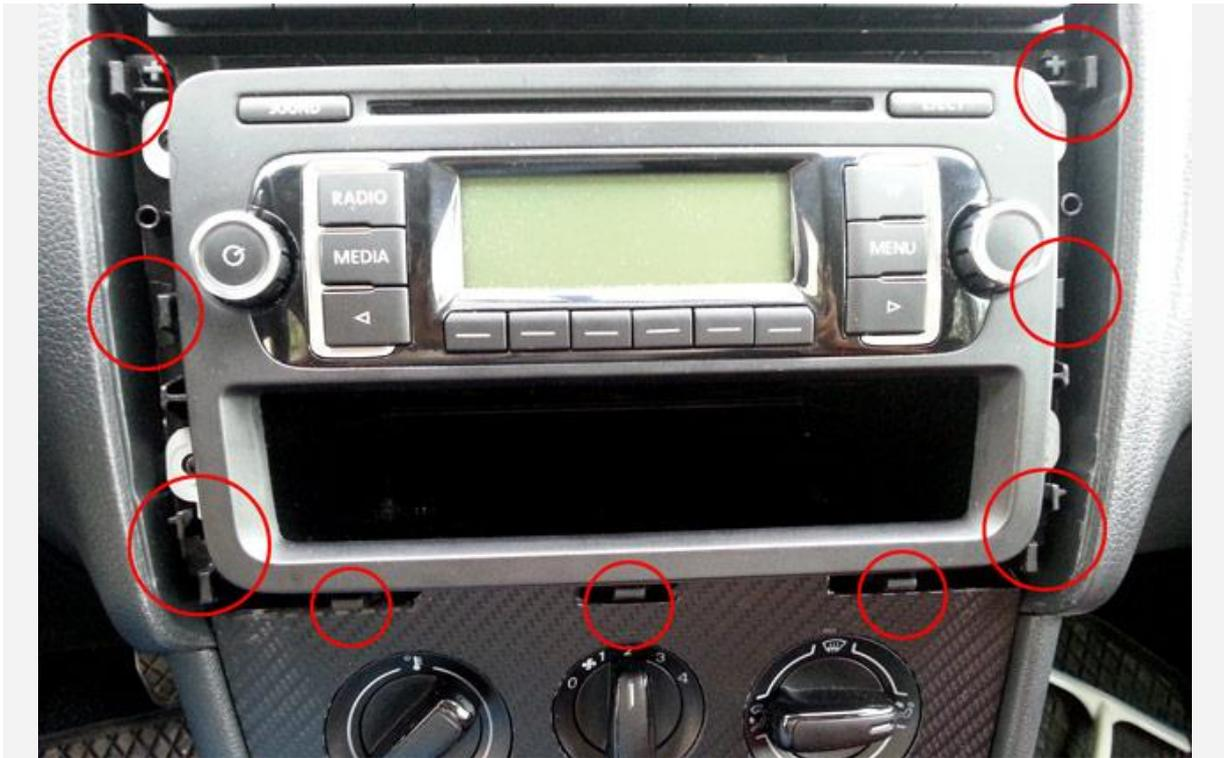
Front view of the car radio with the plastic frame removed. Notice the placement of the clips. The three on the buttons are not very strong, so be careful when you unclips them.
