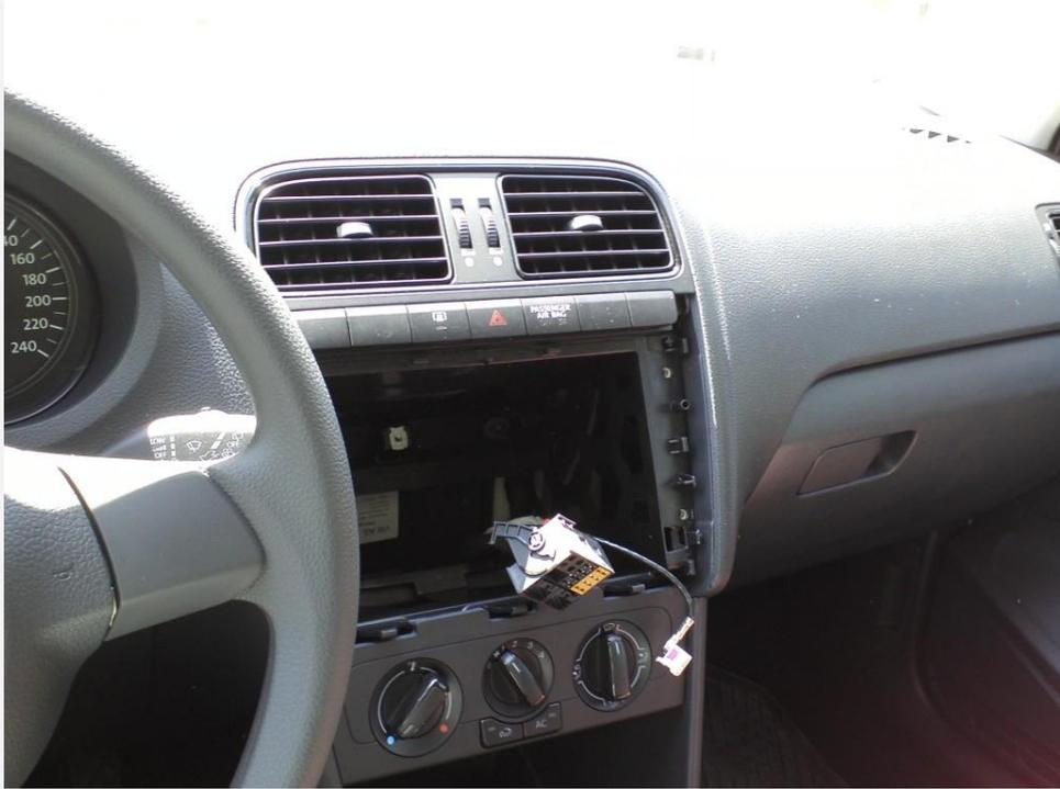
Here you can distinguish the Quadlock (big squared connector) and the small antenna cable (white). Please note that if you have disconnected the Quadlock from the car radio you will need the anti-theft activation code when you turn your radio on.
