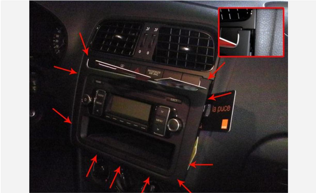
The arrows show where to place your tool in order to reach the clips. Please don't use any screwdrivers because you would scratch the frame and if you make a bad manipulation even the car radio itself.
