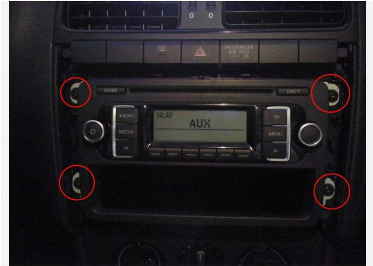
Theses screws can be easily removed with a Torx-Screwdriver (10)
