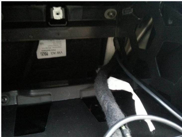
Now you can put the cable along the big Quadlock cable. You can push the cable till it comes out on the bottom of the central console.
