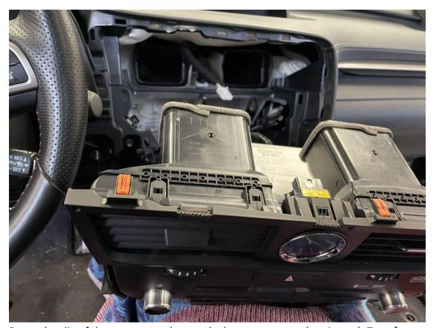
Press the clip of the gray part to loosen the large connector (see image). Transfer the two connectors that are released to the contra connectors.
