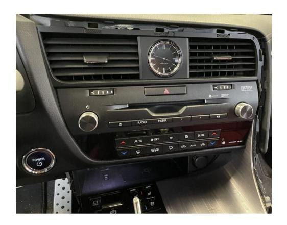
Step 3. Remove the panel to the left of the radio console (unclip)
