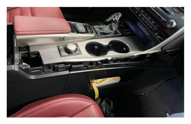
Step 2. Remove the decorative strip from the radio console (unclip)
