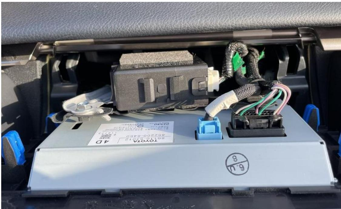
**Step 6. Connect the plugs to radio and display**
