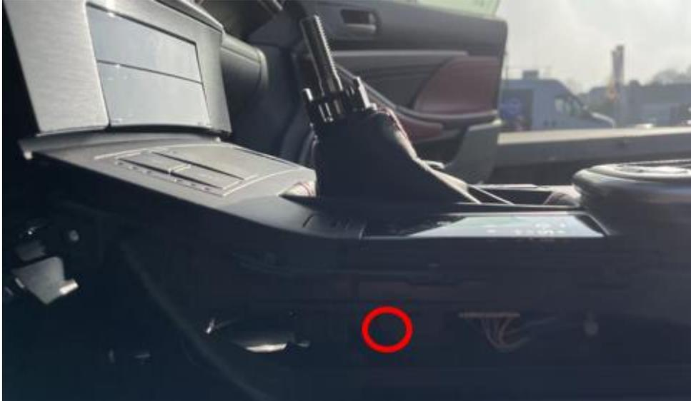
Pull up the top of the center console from the rear and pull it back as far as possible. If necessary, disconnect the plugs to make more space.
