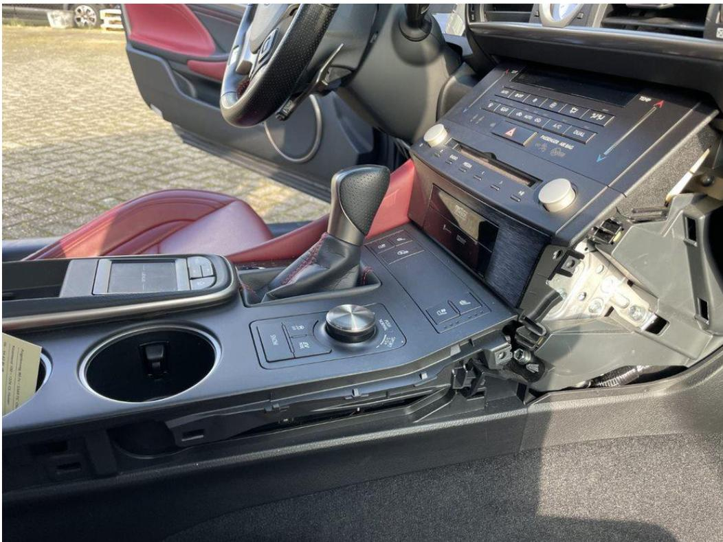
**Step 2. Detach the center console (unscrew and unclip)**
