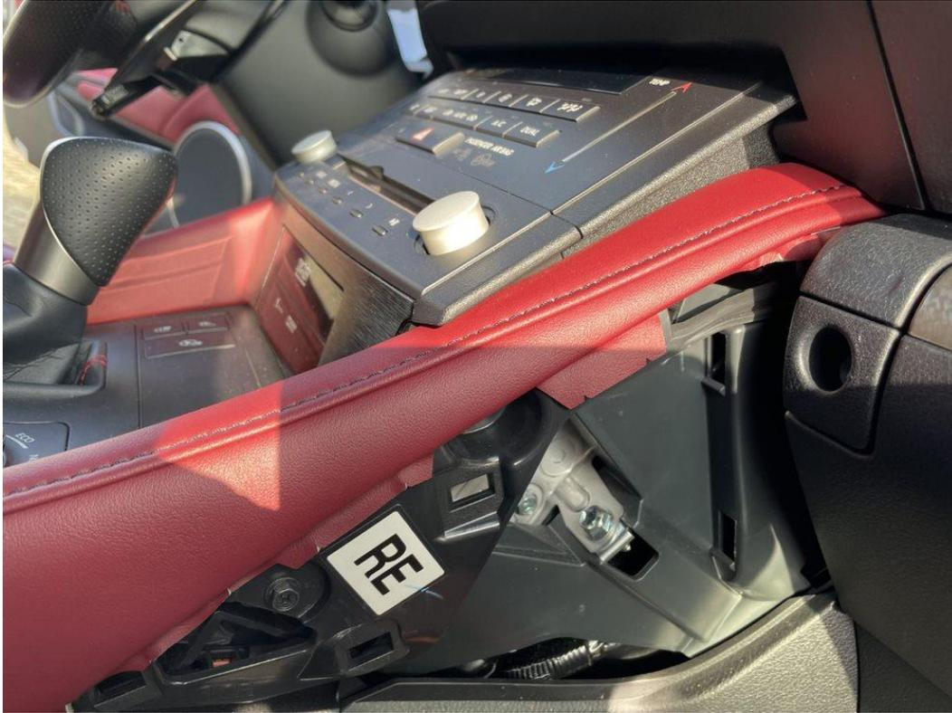
Unscrew both long panels (two screws on each side) and gently stretch the panel from the narrow side and work towards the dashboard. Place the panels in a safe place. If necessary, use removal tools.
