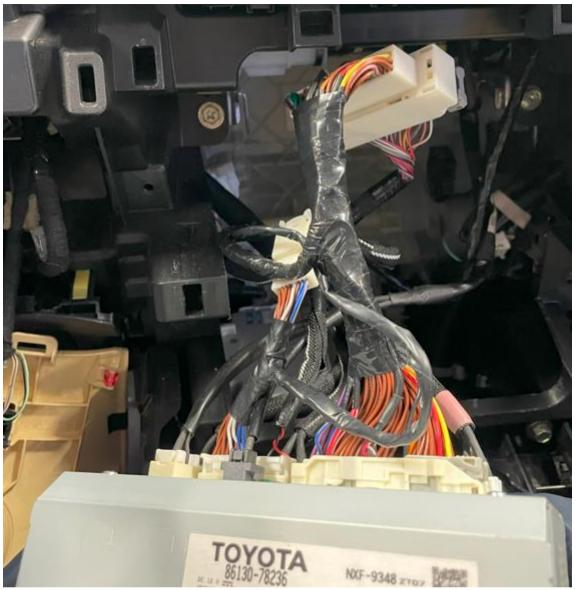
Swap the monitor's blue video plug for the new plug, and then connect the old plug to the new socket. Route the cables to the right compartment.
