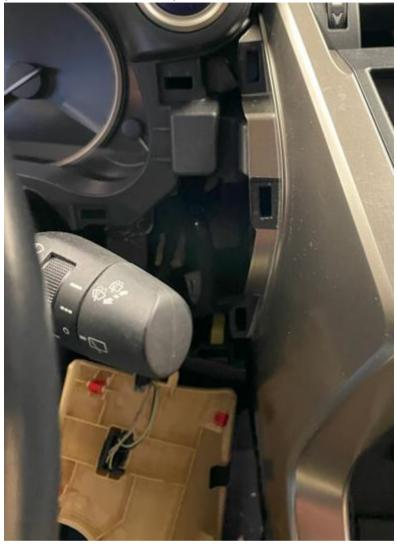
*Step 7. Remove screen panel (click off)* Peel off the panel in front of the display by pulling it up and forward.
