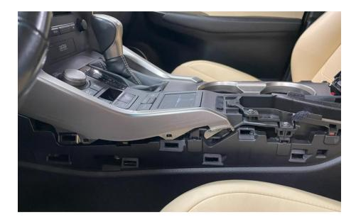
**Step 5.** Remove the front panel on the right (unclip) Pull the front panel up and off at the co-passenger's position.
