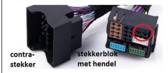
Remove this optical plug by pressing the tab and gently pulling the plug out of the power strip with the orange or green optical cables. Press the optical plug into the same position in the other power strip with lever.
