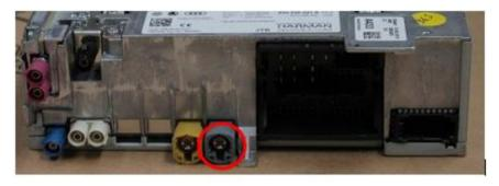
Press the pallet from the grey or pink video connector on the bottom. Very carefully pry a small flat object between the seam if the plug is very tight. Leave the rest of the plugs plugged in. If necessary, cut some tape between the cables so that there is enough freedom of movement to be able to pull the thick cable and the video cable out of the housing.
