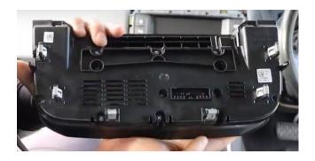
Step 4. Remove the display (screws)
