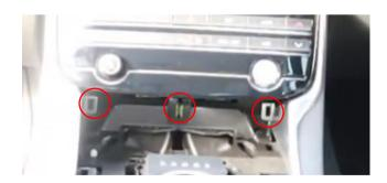
Pull off the air conditioning panel completely. This one is very tight, but it's 6 clips, it's not screwed.
