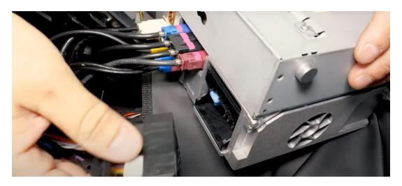
Connect the original plug to the socket of the interface. Push the black power strip back into the radio.
