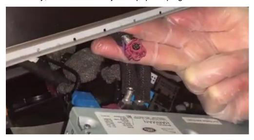
Connect the released video plug to the socket of the other video cable (this can only be done in 1 way).
