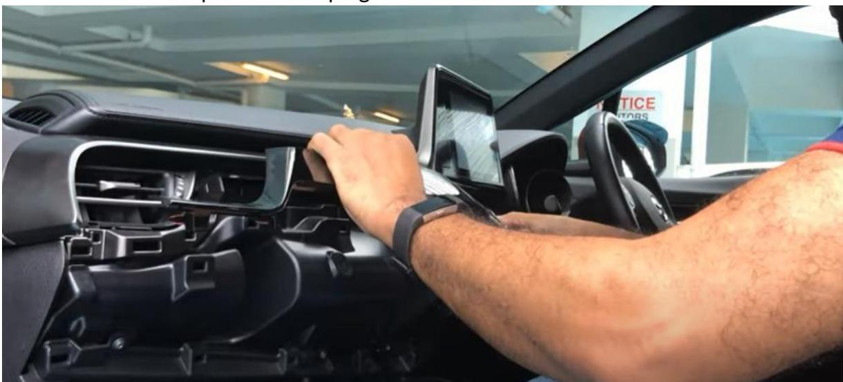
**Step 3. Remove the air vents (unscrew)**
