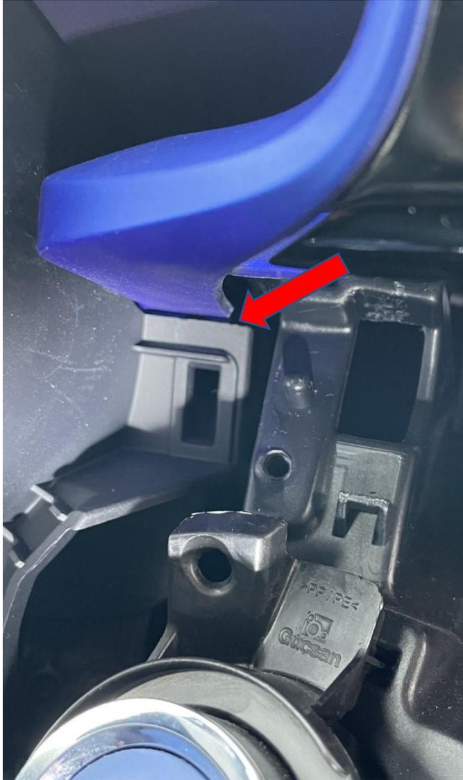
**Step 5. Remove the screen (unscrew)**
