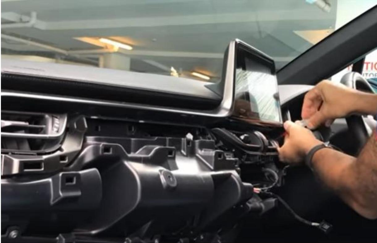
**Step 4. Remove the bezel of the screen (unclip)**
