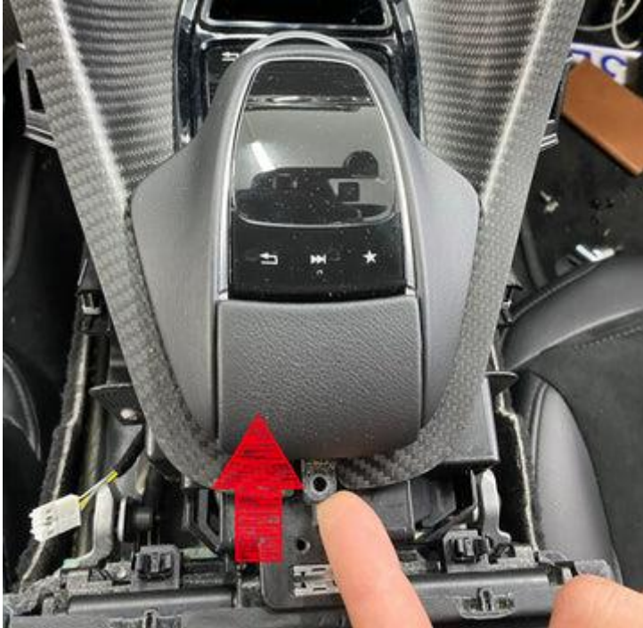
Remove the plastic cover on the knob and the 2 screws.
