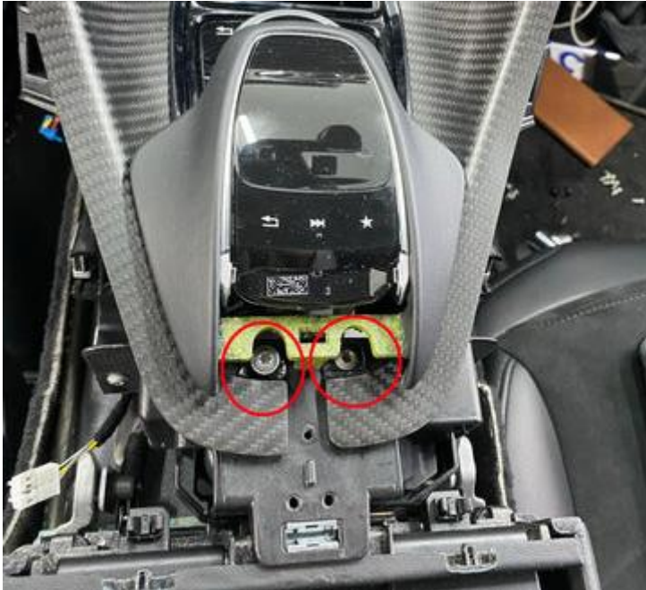
Remove the plastic cover on the knob and the 2 screws.
