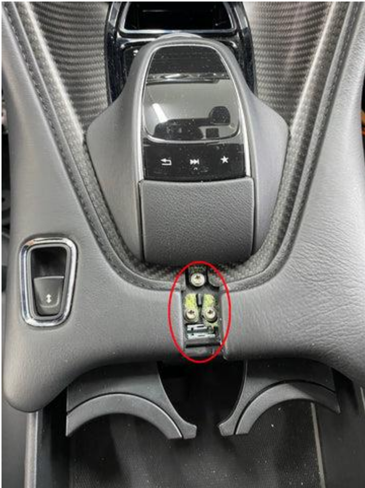
Unclip the small cover under the wheel (joystick) which reveals 3 screws.
