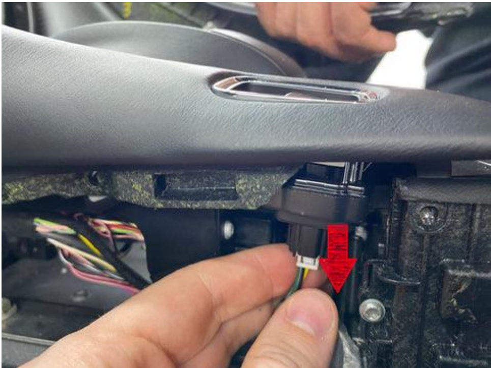
Unclip the small cover under the wheel (joystick) which reveals 3 screws.
