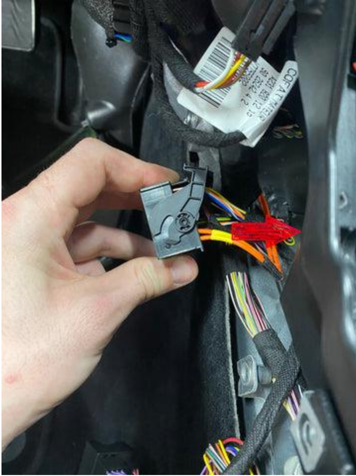
Take the fiber out of the quadlock and reconnect it to the new connector on the host.
